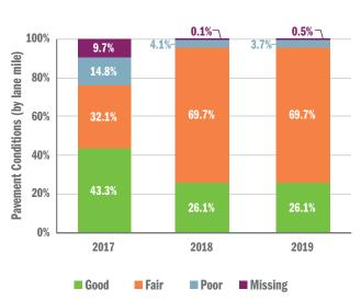
Figure 8.3: Non-Interstate NHS Pavement Conditions, 2017 – 2019 [4654.3 Non-Interstate NHS Lane Miles] (Source: Transportation Planning Board, 2017; includes IRI data only, data excludes sections with bridges, ramps, non-mainline, noninventory direction, planned/unbuilt, unpaved and other types.)
